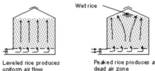
Figure 4. Effect of overfilling a storage bin.
